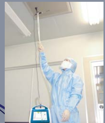
Climomaster™ probe for environmental measurements
